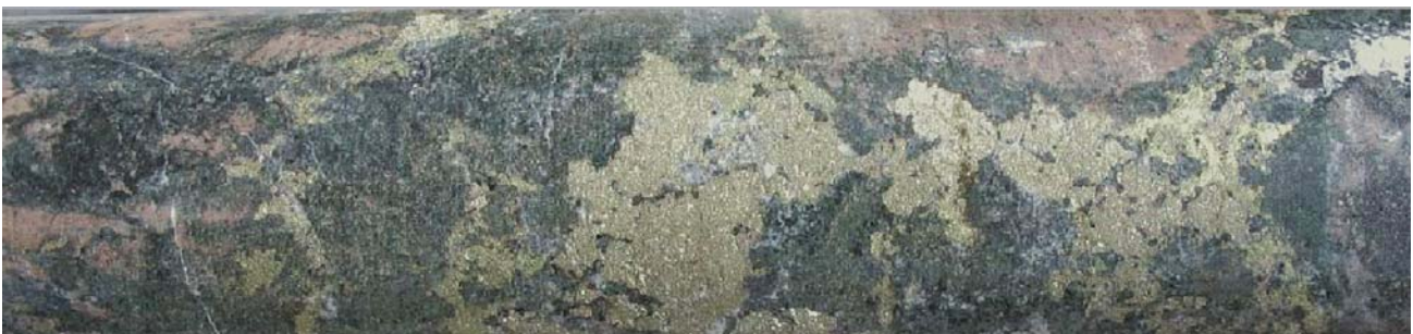
Figure 1 – IOCG style alteration and mineralisation in the Boomara Project (KDD13, 375.6m)
