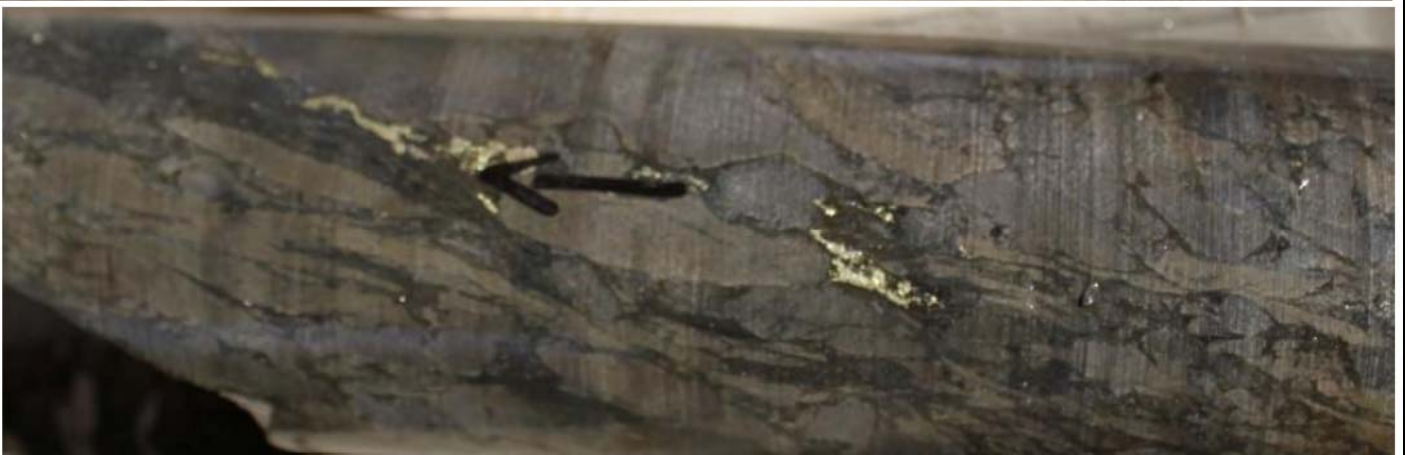
Figure 3: (a) chalcopyrite blebs and stringers with jasperoidal silicification and chloritisation at 635 metres; (b) chalcopyrite bleb at 641 metres; (c) chalcopyrite stringer in breccia at 642 metres
